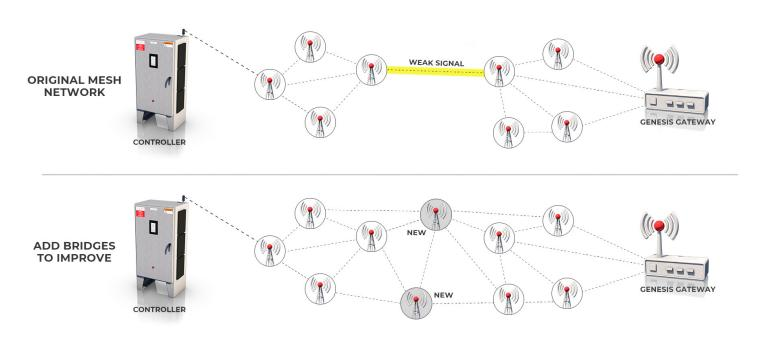
The **Genesis Network** consists of a control room server, a gateway, and a collection of field deployed bridges/nodes that form a wireless mesh communications network. Alternatively, the network can be made via a traditional wired Ethernet network. The Genesis™ Network connects all heat trace panels and controllers to the control room and gives visibility of all assets from a single dashboard and user interface that can be accessed from any browser.
