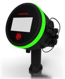
Upgraded Communications: The Duo is Genesis Network native with the built in wireless mesh or wired ethernet. The Duo can also optionally be connected directly to any plant DCS system via Modbus RTU (Modbus TCP will be available in a future update).
